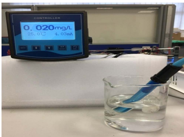
Figure 1. Dissolved ozone analyzer KRDRY-2056.
