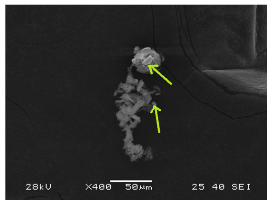
Figure 2. SEM image of rice husk (RH) at 400 \times magnification.
